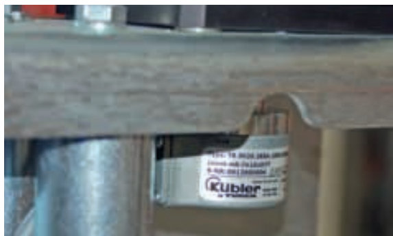
A custom-built encoder with a d-sub connector was designed for Pro Pack's new machine
